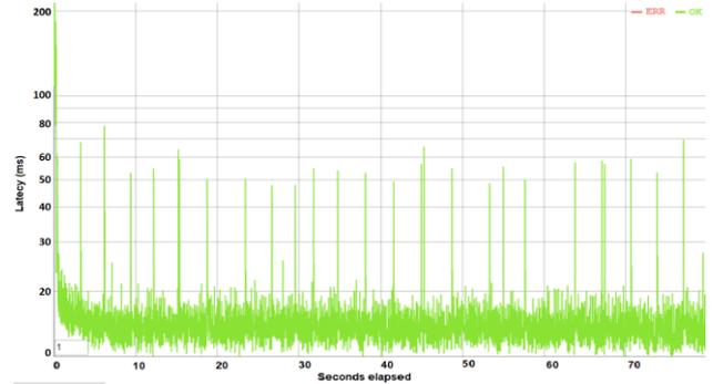
Fig. 5. Load test with sensors data brokering approach.
