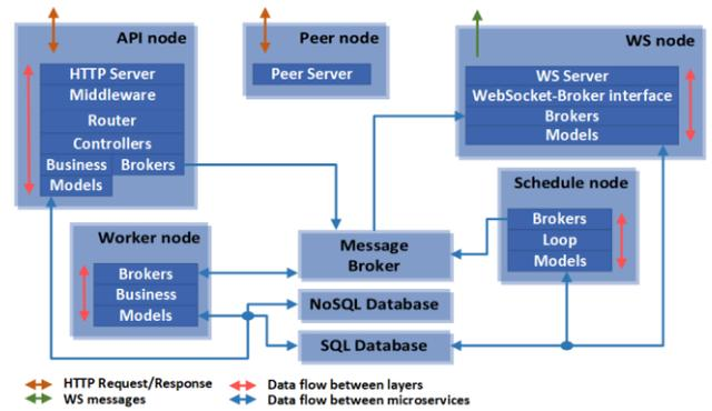
Fig. 3. Cloud microservices architecture.
